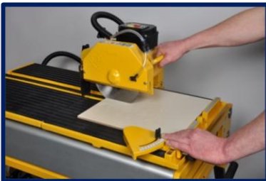
PULL Cuts – Position the tile & pull the cutting block through the tile
