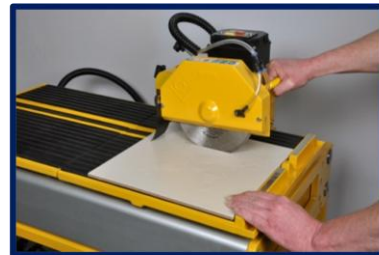
PLUNGE CUTS – Lift the cutting block & position over the tile to cut
