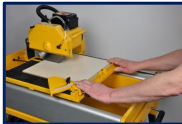
PUSH Cuts – Use the sliding cutting table to push the tile to the blade
